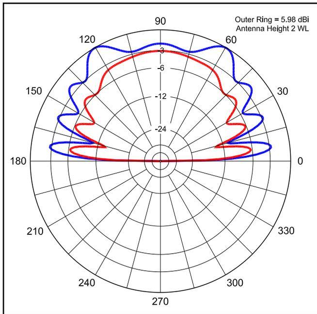
Figure 3—A comparison of elevation patterns for the turnstile-and-screen system (with  $\frac{3}{8}\lambda$  wavelength spacing, shown in blue) and a Moxon pair (shown in red), both at  $2\lambda$  height.
