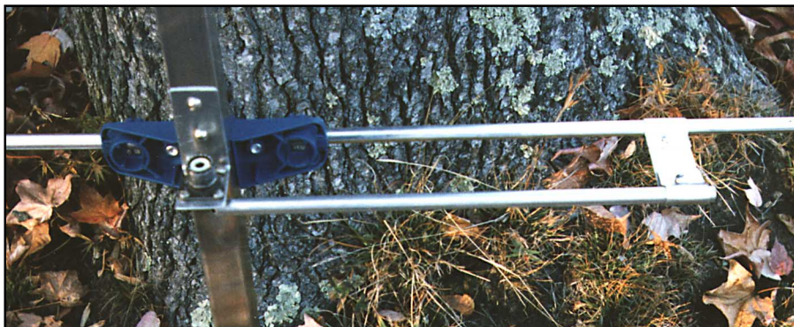
Figure 6—The gamma match and driven element.
