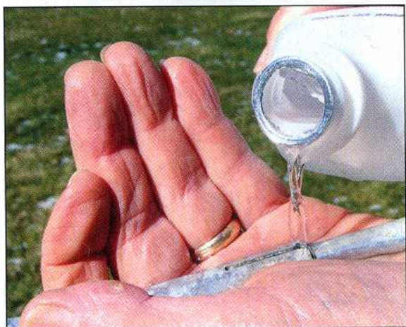
Figure 5 — A little rubbing alcohol applied to the junction of two stuck antenna elements can soften whatever impurities have become lodged between the sections, allowing them to be more easily separated. [Lorraine Wilkinson, W7RFC, photo]
